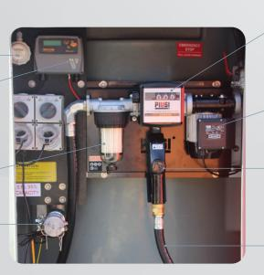
Mechanical fluid meter (digital available with Ranger and Quantum models)
