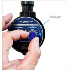
1i. Ensure that the reset interval and drain time knobs are in the "RESET" and "CLOSED" positions. Set your reset interval and drain time according to the tables in Figure 2, then replace the battery box cover.
