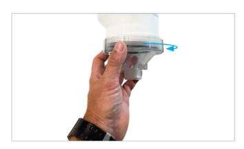
1c. Attach the Electronic Release Valve by first installing the 25mm x 20mm (1" x 3/4") reducing adaptor and washer to the 25mm (1") thread of the screw cap.
